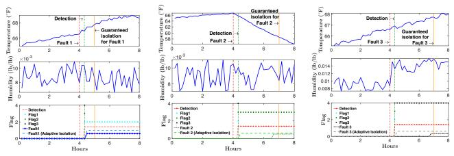
Fig. 3: The outputs (top two rows) of 3 fault scenarios; Detection, isolation and adaptive isolation signals for all faults (bottom row). Flag i is non-zero when the model invalidation problem associated with fault i using the adaptive horizon length is validated. Adaptive isolation occurs when only one Flag is non-zero.
