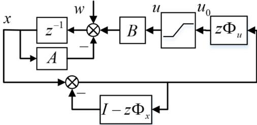
Fig. 4: Closed-loop system under original SLS controller with saturation
