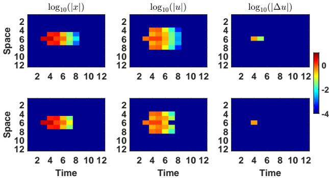
Fig. 7: Simulation of naive SLS with saturation (top) and SLS with saturation compensation (bottom).
