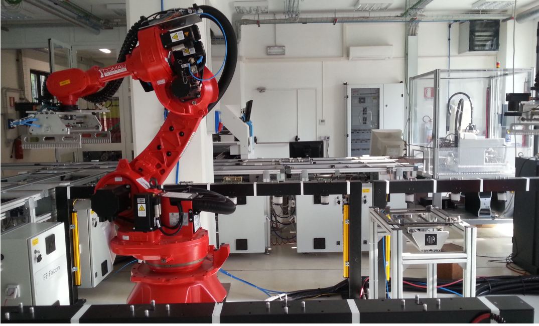
Fig. 1. Laboratory de-manufacturing plant at the National Research Council in Milano ([8]), showing the loading/unloading node with a manipulator, and the transportation nodes and a machine node in the background.
