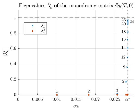
Fig. 2. Eigenvalues of the monodromy matrix  $\Phi_k(T, 0)$  of  $F_k(\cdot)$  defined in (10) for  $\alpha = \alpha_k$ . The iteration number  $k$  is written near the eigenvalue  $\lambda_k^1$ . As  $\alpha_k$  goes to  $\alpha^*$ , the eigenvalue  $\lambda_k^1$  of  $\Phi_k$  converges to the unit circle. At  $\alpha^*$ ,  $F_{\alpha^*}(\cdot)$  is not exponentially stable anymore and have neutral trajectories.
