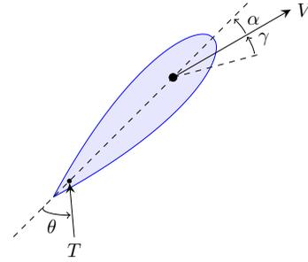
Fig. 5. Description of the vectored thrust flying wing model.  $V$  is the velocity vector,  $T$  is the thrust,  $\theta$  is the direction of the thrust vector in the flying wing frame.
