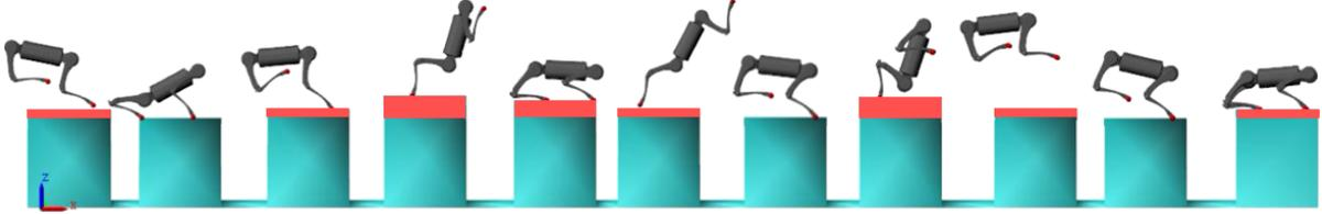
(b) **Case II - Random distance and random height perturbations.** The stepping stone are randomly placed with step length in (60 : 90)cm. The gap heights vary randomly between  $-6\text{cm}$  to  $+5\text{cm}$ , which are unknown to the robot
