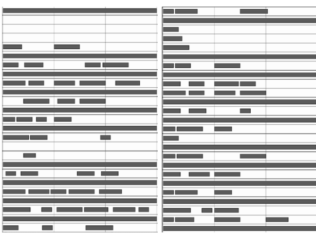
Fig. 5. Two individuals of the left Pareto front from Fig. 4. It can be seen that if waiting time for trucks is the main objective, then at least one truck has been assigned to each gate and trucks are docking to gates very early in general (right chart). On the other extreme if mainly the transportation volume inside of the terminal is considered then some of the gates are not used at all while some - probably generally good gates - are very crowded and some trucks are assigned to gates on a very late time slot (left chart)
