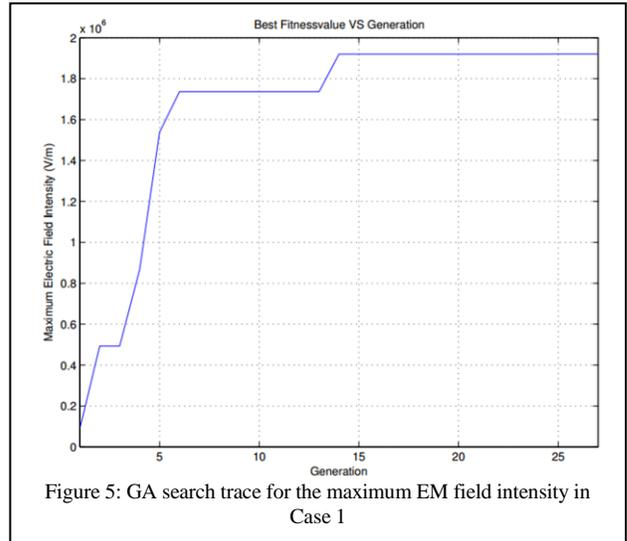
Figure 5: GA search trace for the maximum EM field intensity in Case 1
