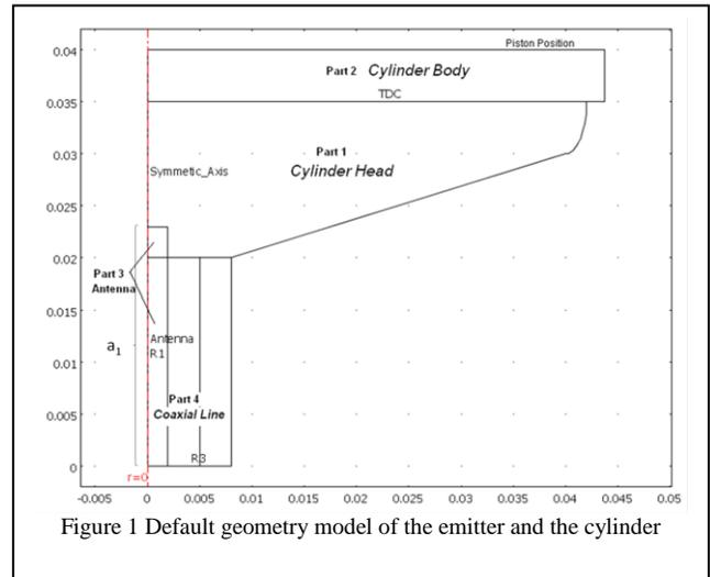
Figure 1 Default geometry model of the emitter and the cylinder
