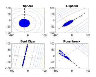
Fig. 1. Sampling of points (blue) within  $[-100, 100]^2$  and new reference system (dashed black lines) for shifted and rotated Sphere, Ellipsoid, Bent Cigar, and Rosenbrock functions below the threshold values  $10^3$ ,  $3 \times 10^4$ ,  $10^6$ , and  $5 \times 10^3$ , respectively.
