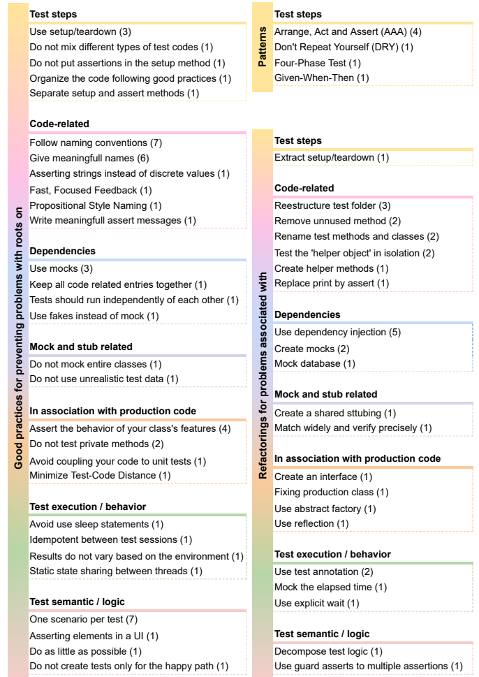
Fig. 7: Suggestions of patterns for code organization, good practices, and test code refactorings for preventing and fixing test smells.
