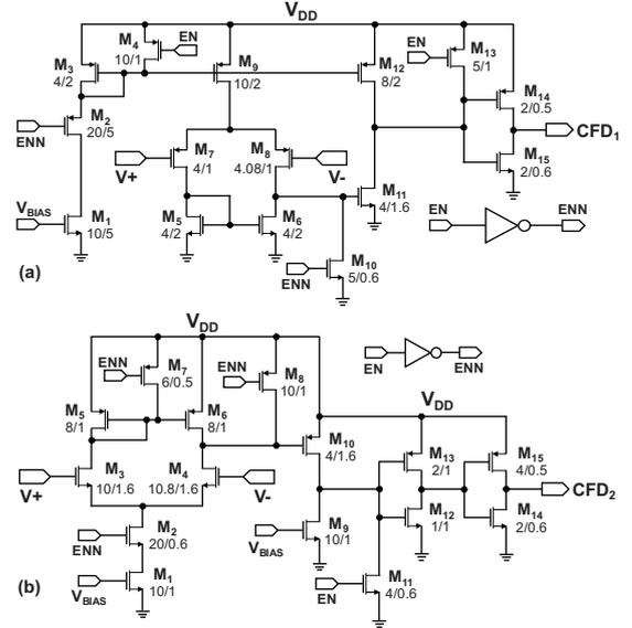
Fig. 6. Schematics of (a) charge flipping detector-1 ( $CFD_1$ ) and (b) charge flipping detector-2 ( $CFD_2$ ).
