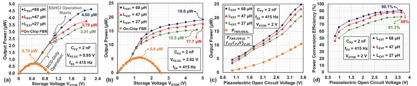
Fig. 8: (a, b) Measured output power by SSHCI circuit compared to on-chip full-bridge rectifier (FBR) with different piezoelectric open circuit voltage levels  $V_{PZ,OC}$ , and (c) ideal FBR, and (d) power conversion efficiency of the operation.
