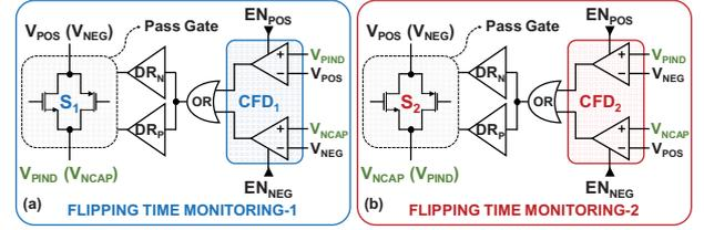
Fig. 5. Flipping time monitoring configurations established for (a)  $S_1$  and (b)  $S_2$  switching operations.
