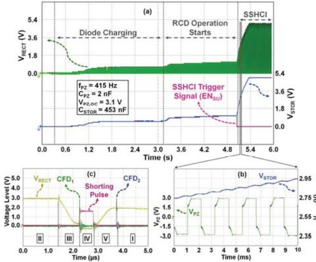
Fig. 7: Measured waveforms of SSHCI circuit illustrating (a) start-up, (b) charging, and (c) control signals generated during voltage flip operations.
