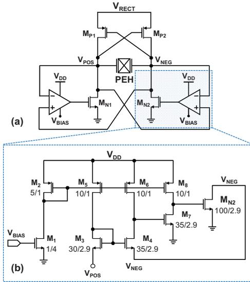
Fig. 4. (a) Implementation of negative voltage converter (NVC) and (b) the comparator utilized inside NVC circuit.
