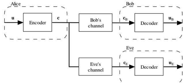
Fig. 1. Block scheme of a wire-tap channel.
