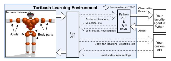
Fig. 2. Overview of the Toribash Learning Environment (ToriLLE). ToriLLE uses Toribash's Lua scripts to communicate with outside controllers over TCP/IP. For each turn, game sends an observation vector to the controller. Controller replies to this by sending a list of joint states to be executed, and Toribash progresses by one turn.
