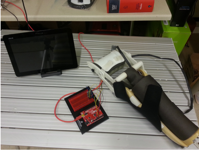
Fig. 1. The robotic system for rehabilitation of hand function, including a Hand Mentor (right), microcontroller and Bluetooth (middle), and tablet (left).
