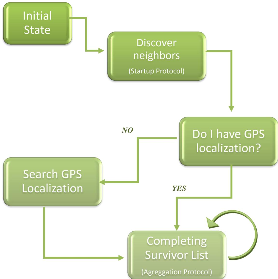
*Figure III.22 Self-model designed to configure the rules of the Survivor's reasoning*
