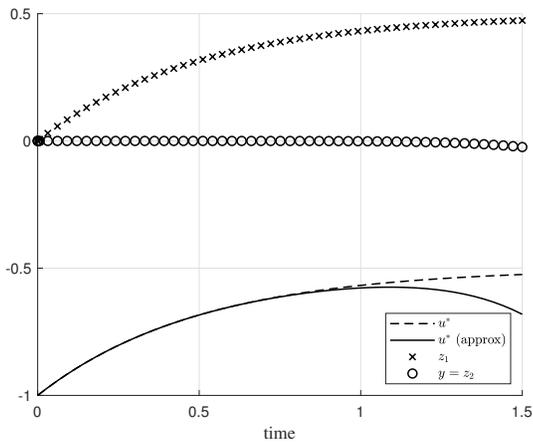
Fig. 1. Approximate zero dynamics of the CSTR system in Example 4.3 using only knowledge of the plant’s generating series.
