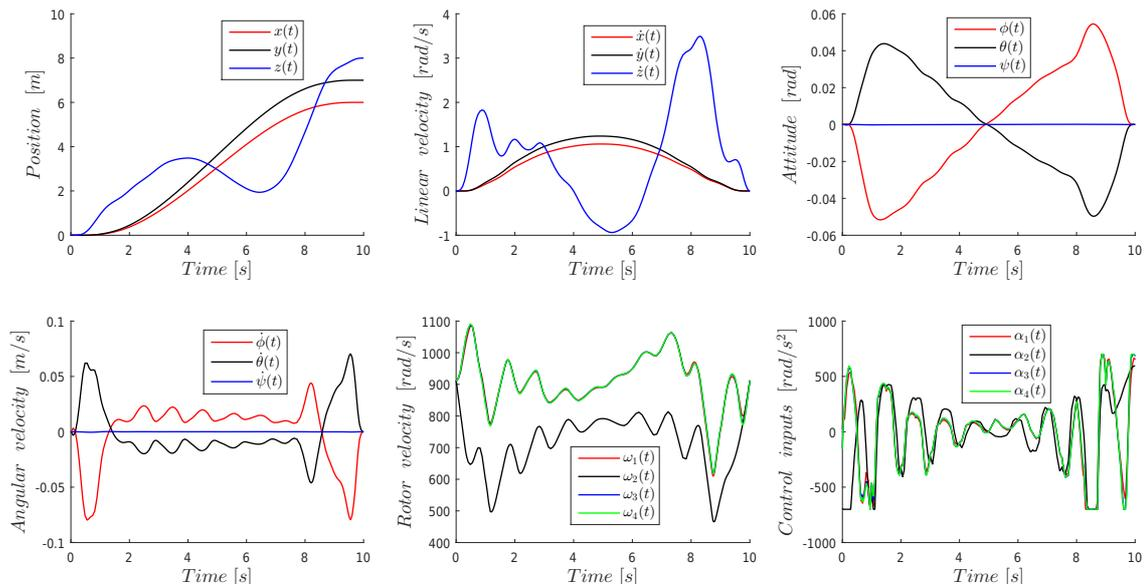
Fig. 3. Time evolution of the state variables  $x_1(t), x_3(t), x_5(t)$  quadrotor position,  $x_2(t), x_4(t), x_6(t)$  linear velocity,  $x_7(t), x_9(t), x_{10}(t)$  quadrotor attitude,  $x_8(t), x_{10}(t), x_{12}(t)$  angular velocity,  $x_{13}(t), x_{14}(t), x_{15}(t), x_{16}(t)$  rotors velocity and control inputs  $\alpha_1, \dots, \alpha_4$  rotors acceleration, relative to the path from  $\mathbf{x}_0$  to  $\mathbf{x}_f$ .
