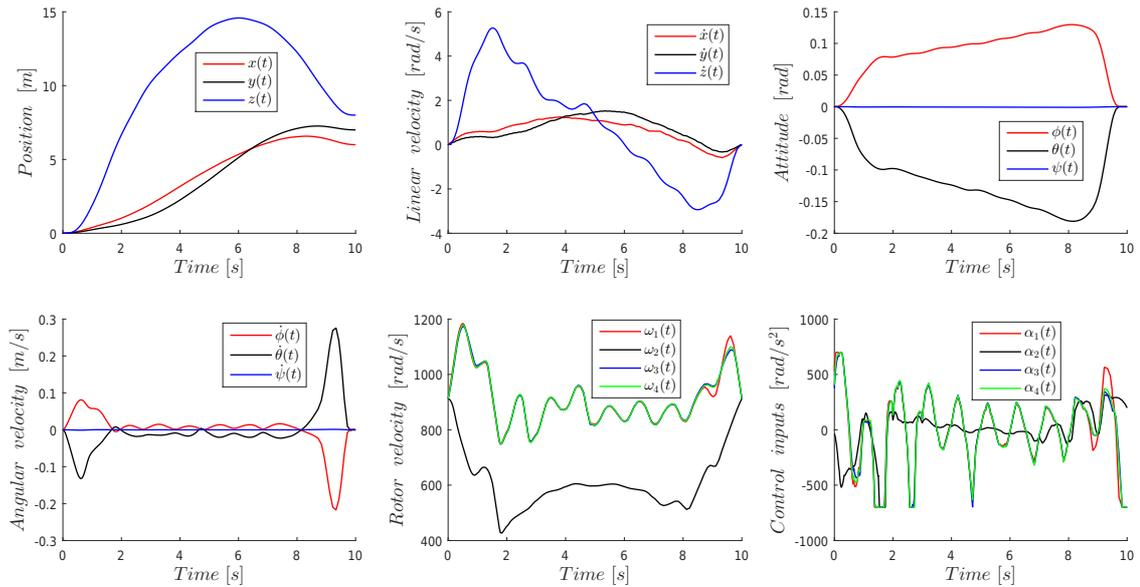
Fig. 5. Time evolution of the state variables  $x_1(t), x_3(t), x_5(t)$  quadrotor position,  $x_2(t), x_4(t), x_6(t)$  linear velocity,  $x_7(t), x_9(t), x_{10}(t)$  quadrotor attitude,  $x_8(t), x_{10}(t), x_{12}(t)$  angular velocity,  $x_{13}(t), x_{14}(t), x_{15}(t), x_{16}(t)$  rotors velocity and control inputs  $\alpha_1, \dots, \alpha_4$  rotors acceleration, relative to the path from  $\mathbf{x}_0$  to  $\mathbf{x}_f$  under wind gust conditions
