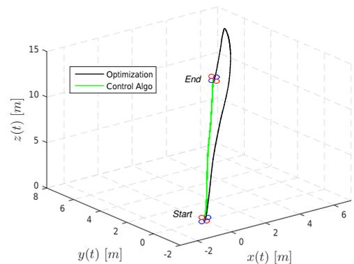
Fig. 7. Energy-efficiency 3D trajectory under wind gust conditions
