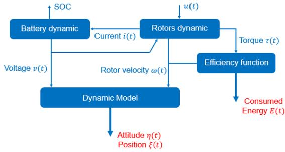
Fig. 1. Power loss model for quadrotor aerial vehicle
