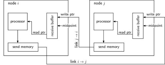
Figure 1: Two nodes showing the receive buffers as part of the links.
