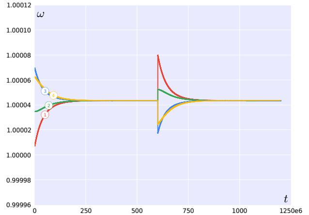
Figure 4: Frequency behavior as a function of time. The reframing occurs at about  $t = 600\text{ns}$ . Simulations were performed using the *Callisto* [4] simulator with a detailed frame-accurate model of bittide. Traces on the graph are labeled with the corresponding node number.
