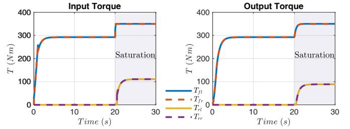
Fig. 4. Actuator Inputs/Outputs using DCKFCA in Scenario 2.
