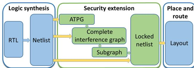
Fig. 7. Design flow with the security extension module.
