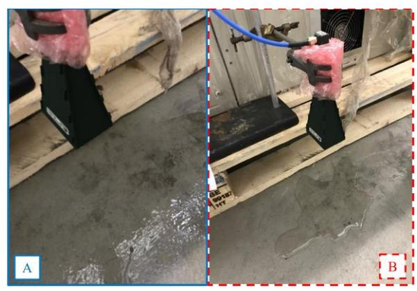
Figure 5. A) A wet cloth was applied to dampen the test area, note light surface sheen due to moisture. B) ~20 ml of water deposited in the sensor field of view.
