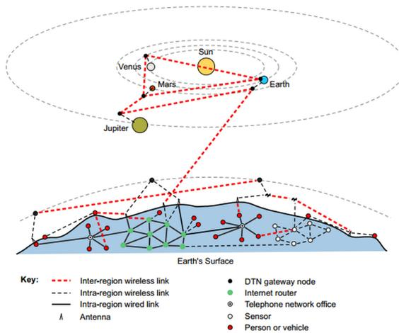
Fig. 1. Heterogeneous Delay Tolerant Network Example [15].
