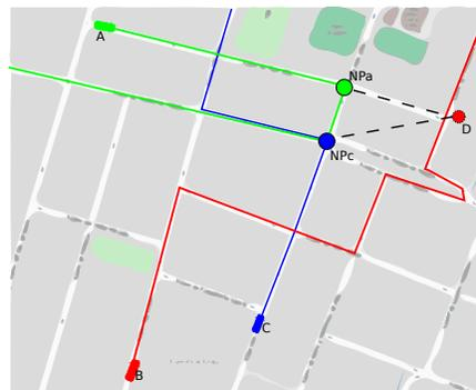
Fig. 12. Calculation of the  $NP$  in GeOpps. Although  $NP_B$  is closer to the destination than  $NP_A$  and  $NP_C$ , A and C nodes are probably better forwarding nodes, since they will reach their NPs faster than B.
