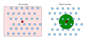
Fig. 22. The basic principle of the SD based MIMO detectors. In short, it solves the problem of finding the "closest" lattice point to a given vector y in the skewed and rotated (caused by the MIMO channel) lattice Hs.
