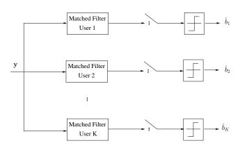
Fig. 16. An implementation example of the MF detector for synchronous CDMA systems employing BPSK modulation.
