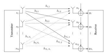
Fig. 13. Schematic of VBLAST-style SDM-MIMO systems communicating over flat fading channels.
