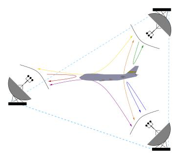
Fig. 30. Conceptual illustration of MIMO radar systems.
