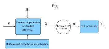
Fig. 25. The basic principle of the SDPR based MIMO detectors.
