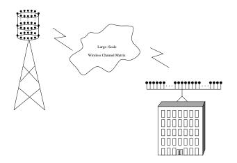
Fig. 27. An example of Type-I (point-to-point) LS-MIMO systems.
