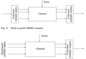
Fig. 9. MIMO multiple-access channel.
