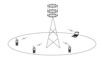
Fig. 28. An example of Type-II (multiuser) LS-MIMO systems.
