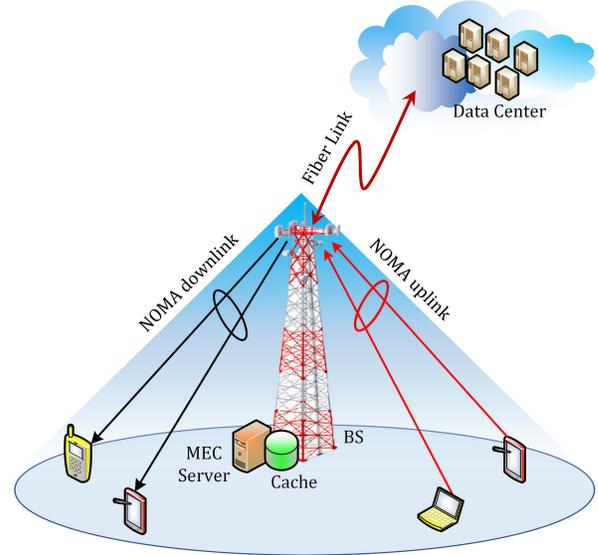
Fig. 11: Basic architecture of a cache-aided NOMA MEC network. User's devices offload computational tasks to cache and MEC-aided BS [188].
