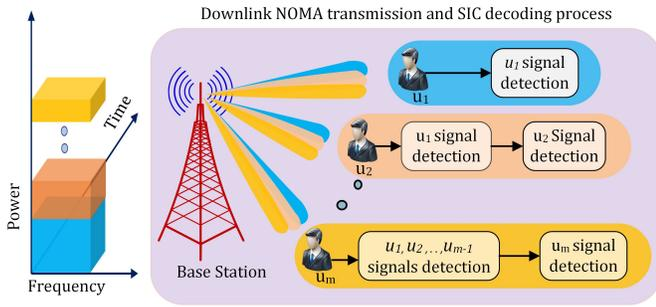
Fig. 3: Power distribution strategy for PD-NOMA. The transmitter allocates maximum power to user  $u_1$  with the weakest channel and minimum power to user  $u_m$  with the strongest channel.  $u_1$  decodes its own signal directly, and  $u_m$  first decodes signal of  $u_1, u_2, \dots, u_{m-1}$  then its own signal.
