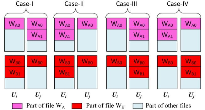
Fig. 4: Different cache status of  $U_i$  and  $U_j$  requested file  $W_{fn}$ ,  $f \in \{A, B\}$ ,  $n \in \{0, 1, 2\}$ . For all four cases, the file portion  $W_{f0}$  and  $W_{f2}$  are cached and uncached, respectively. Thus, the transmitter never transmits  $W_{f0}$  but always needs to transmit  $W_{f2}$  [85].
