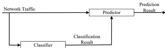
Fig. 19. Feed forward structure for traffic prediction.
