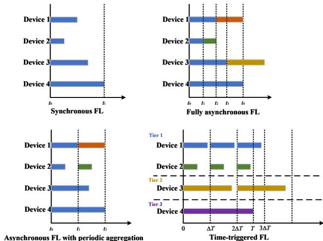
Fig. 10. Illustration of synchronous FL, fully asynchronous FL, asynchronous FL with periodic aggregation, and time-triggered FL.
