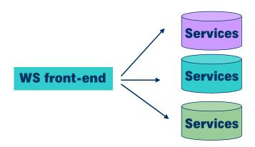
Figure 3: A Web Service composed of a front end and three back-end services that supply content.
