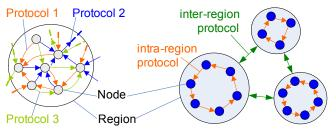
Figure 5: QuickSilver amortizes costs over many groups. Lacking such an approach, chaos can occur, as is seen on the left, where each group builds its own recovery infrastructure (here, a tree-like overlay).
