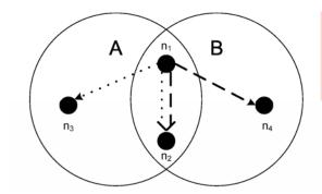
Figure 2: Ricochet introduces "lateral error correction", whereby error correction data is proactively multicast by other receivers in overlap regions. Lost data is often recovered before the sender can detect the loss.
