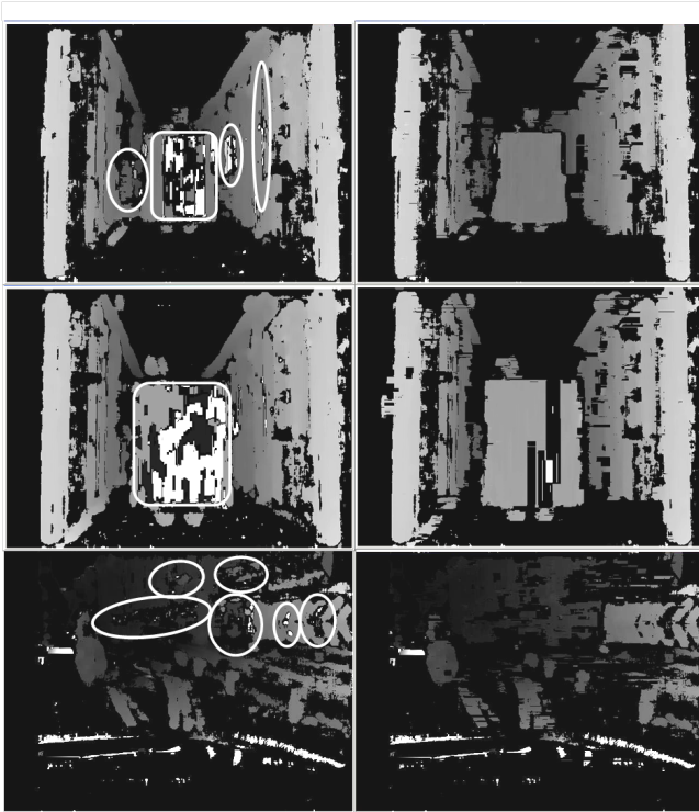
Figure 8. Left: The initial depth map calculated with a state-of-the-art block matching algorithm. Right: The fused result. Top: 14cm periodic pattern at 4m distance. Middle: 8cm periodic pattern at 3.5m distance. Bottom: Urban scene. A camera with focal length f=510 pixels and 9cm baseline was used.
