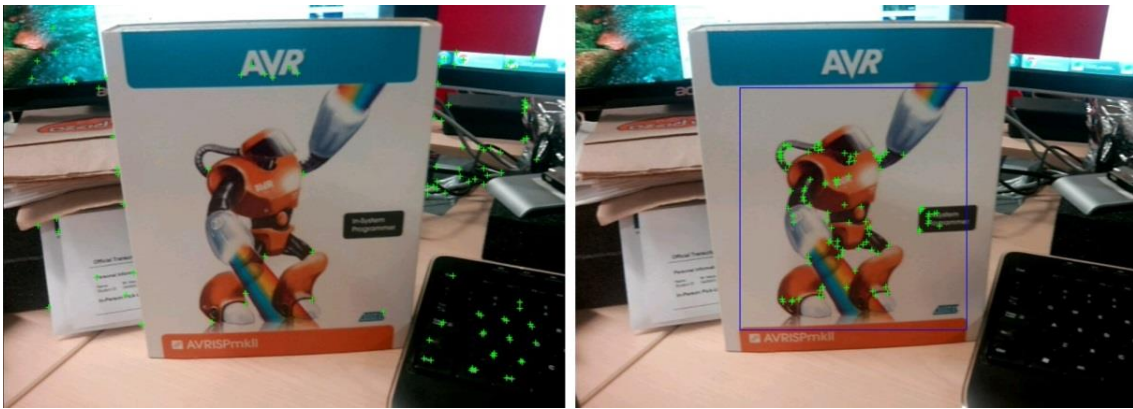
Figure 3.9 - Left: No map is found, features (green crosses) are extracted from the entire image. Right: Features are extracted only from within the map ROI (blue rectangle). For clarity, only 100 features are extracted for this example.
