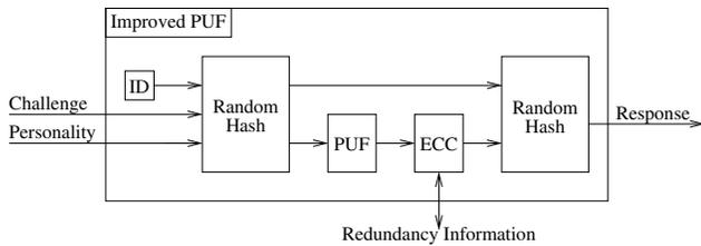
**Figure 1. Using control to improve a PUF.**
