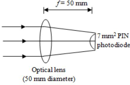
Fig 3: Receiver optics system
