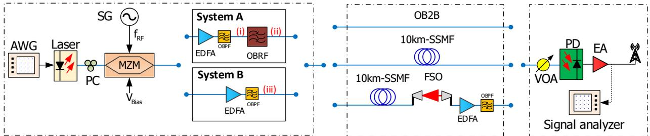
Figure 1. Experimental setup of a DML data signal modulation, carrier suppression and RoF and RoFso transmission. AWG: arbitrary waveform generator, PC: polarization controller, MZM: Mach-Zehnder modulator, SG: RF signal generator, EDFA: erbium doped fiber amplifier, OBPF: optical bandpass filter, OBRF: optical band-rejection filter, OB2B: optical back-to-back, SSMF: standard single mode fiber, FSO: free space optics, VOA: variable attenuator, EA: electrical amplifier, PD: photodetector.
