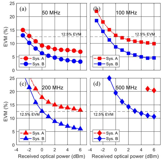
Figure 4. Error vector magnitude (EVM) of System A (Qbias) and System B (CS) for different signal bandwidths for optical back-to-back (OB2B). (a) 50 MHz, (b) 100 MHz (c) 200 MHz and (d) 500 MHz.
