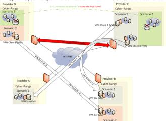
The aforementioned solution seems particularly simple to be used within a commercial federation approach: a simple, replicable VPN VM can be developed and can be easily configured depending on the characteristics of each federated cyber range. Within the ECHO H2020 project, after an initial analysis and subsequent tests, this approach was adopted to develop ECHO Federated Cyber Range system (E-FCR).
