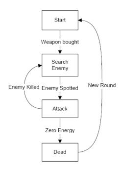
Figure 2. A prototypical FSM for a bots
