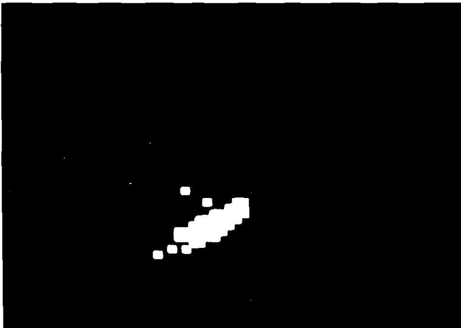
Figure 9: Detection of animate motion. The camera is translating to the left, which means that all the objects in the scene are apparently moving to the right with velocities that depend on their depth. The waving hand, however, can still be detected. The procedure runs in real time (10 frames/sec).
