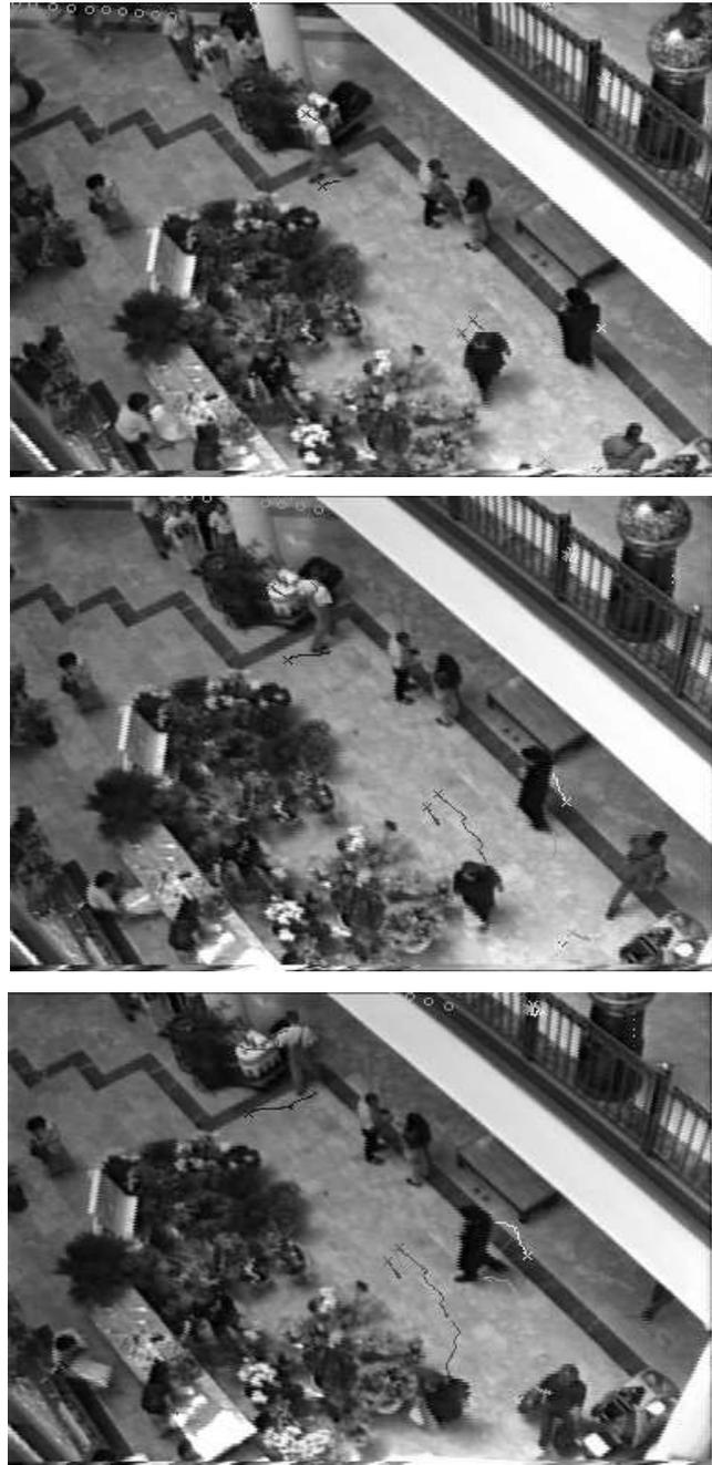
Figure 3. Three frames from a long sequence, taken with a downward moving camera while the people in the scene are moving in different directions. There are 60 frames between the first picture (top) and the last one (bottom); still, 3 figures are reliably tracked, and the tracking is very stable, as indicated by the faint trajectories in black and white (see demonstration in <http://www.cs.huji.ac.il/~daphna>).
