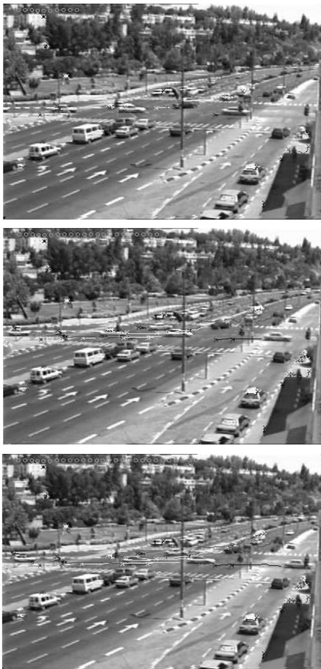
Figure 4. Three frames from another long sequence, taken by a non-stabilized camera in a traffic intersection. The cars which turned to the left changed their 2D projection non-rigidly. There are 60 frames between the first picture (top) and the last one (bottom). The computed trajectories are shown with faint white lines (see demonstration in <http://www.cs.huji.ac.il/~daphna>).
