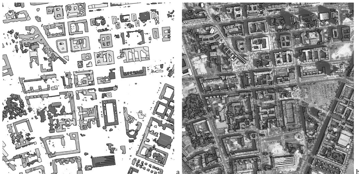
Figure 5. Berlin results of automatic building extraction: (a) the polygonal approximation result superimposed on the DEM composed by all the extracted objects above the ground (small components are then discarded). (b) the final orthogonalized model superimposed on the ortho-image of the scene. Note that the model describes well the main structures of the buildings.
