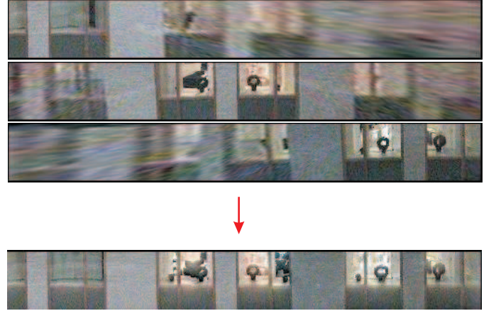
Fig. 6. Final textures of walls are generated by blending multiple textures generated from single panoramic images. Shown here are three of ten textures which are fused into a single texture.
