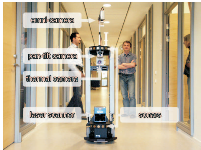
Fig. 1. Robotic platform for security guard with sensors marked. The laser range scanner and the omni-directional camera is used to build a 3D model of the robot's operation environment.
