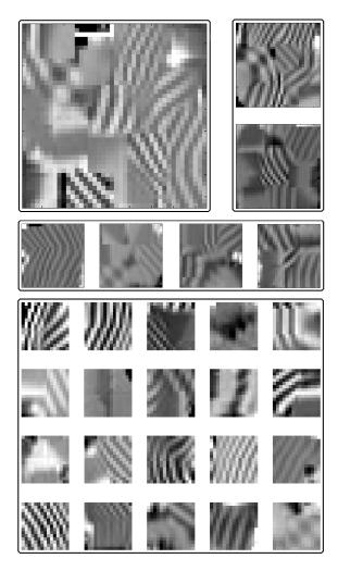
Figure 7. 1, 2, 4 and 20 epitomes learned on the barbara image for the same parameters. They are of sizes 42, 32, 25 and 15 in order to keep the same number of elements in  $\mathbf{D}$ . They are not represented to scale.
