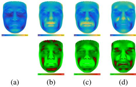
Figure 6: Reconstruction error heatmaps of different methods on the UHDB31 database: (a) *UH-E2FAR*, (b) *RSNIEF*, (c) *RSN*, and (d) *UH-2FCSL*. The top row illustrates the spatial distribution of RMSE on the face and the bottom row illustrates the differences in RMSE between our approach *UH-E2FAR* and other approaches (green indicating our method has smaller RMSE, red indicating our method has larger RMSE, and color intensity indicating the magnitude of the difference).
