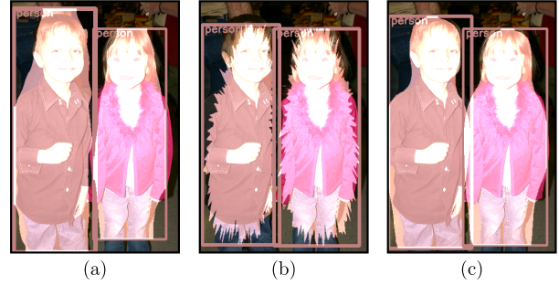
Figure 1: Testing direct regression to shape on a validation image from PASCAL VOC [11] using (a) binary shape masks, (b) radial vectors, and (c) a learned shape embedding.
