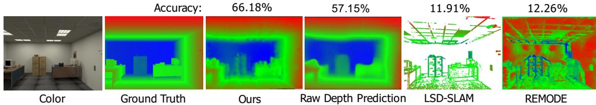
Figure 4. Comparison in terms of depth map accuracy and density among (from the left) the ground-truth, a refined key-frame from our approach, the corresponding raw depth prediction from the CNN, the refined key-frame from LSD-SLAM [4] with bootstrapping and estimated dense depth map from REMODE [23], on the (*office2*) sequence from the *ICL-NUIM* dataset [8]. The accuracy value means correctly estimated depth density on this key-frame.
