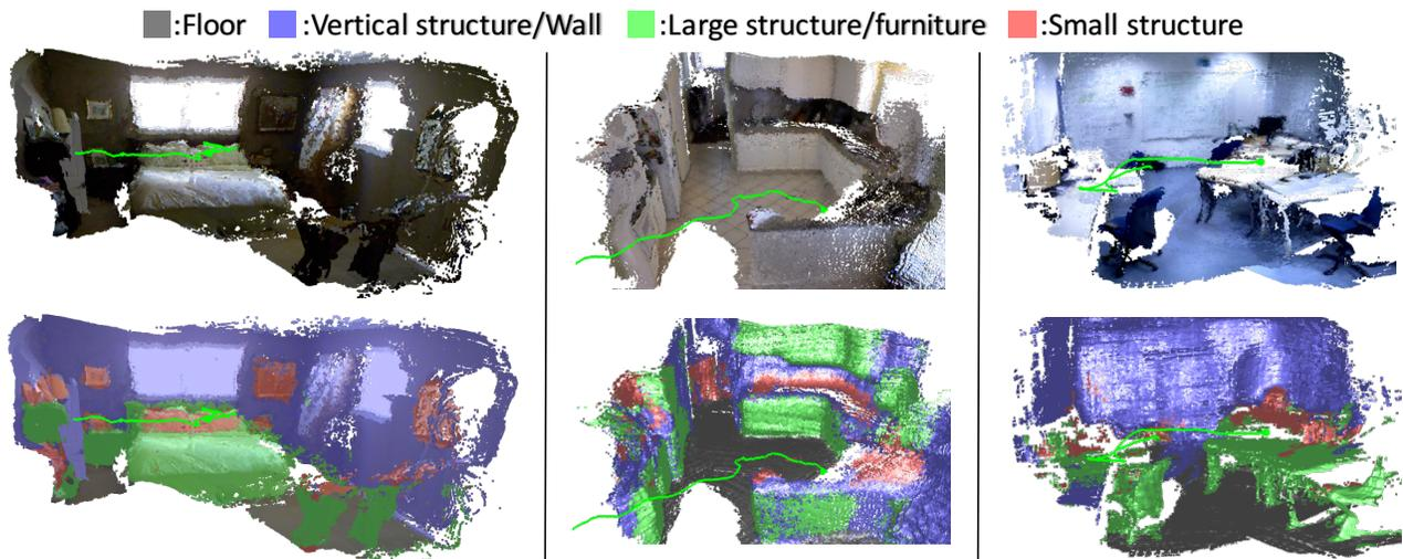
Figure 6. The results of reconstruction and semantic label fusion on the office sequence (top, acquire by our own) and one sequence (*kitchen\_0046*) from the *NYU Depth V2* dataset [25] (bottom). Reconstruction is shown with colors (left) and with semantic labels (right).
