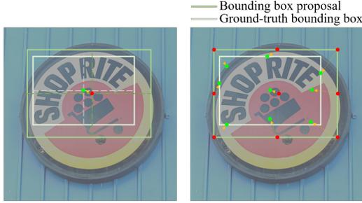
Figure 3. The comparison between conventional RPN (left) and Adaptive-RPN (right). The proposed Adaptive-RPN adaptively regresses the offsets to pre-defined points. Predicted bounding box is generated by bounding the spatial extend of refined points. Red points are pre-defined points in current bounding box proposal (e.g. center point in conventional RPN and pre-defined points  $P$  in Adaptive-RPN), and green points are refined points. The yellow dotted lines indicate the regressed offsets.
