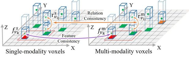
Figure 6. Our sparse-voxel distillation encourages voxel-feature consistency between the single- and multi-modality SSDs in two aspects: voxel features (purple) and voxel relations (orange).
