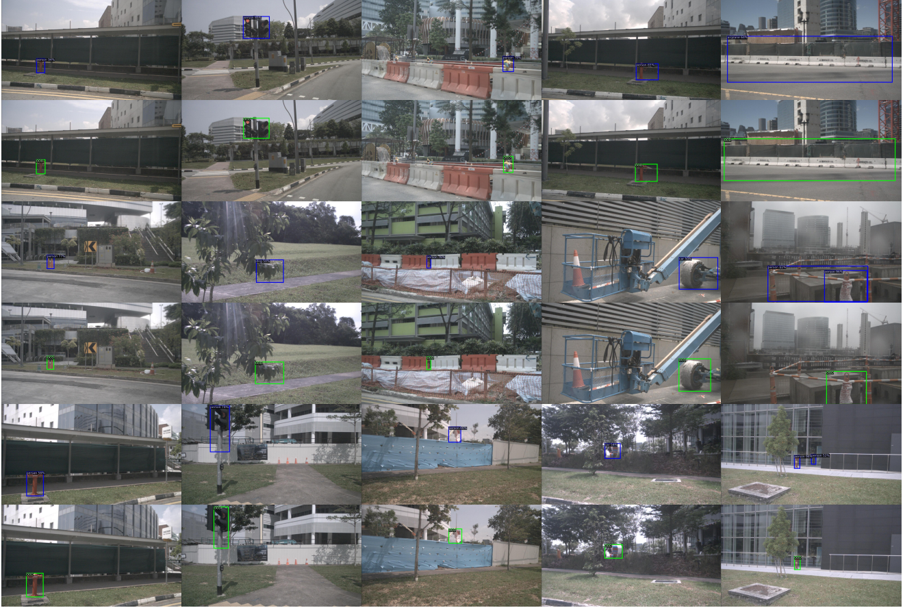
Figure 10. Additional visualization of detected objects on the OOD images (from nuImages) by a vanilla Faster-RCNN ( top ) and STUD ( bottom ). The in-distribution is Youtube-VIS dataset. Blue : Objects detected and classified as one of the ID classes. Green : OOD objects detected by STUD, which reduce false positives among detected objects.
