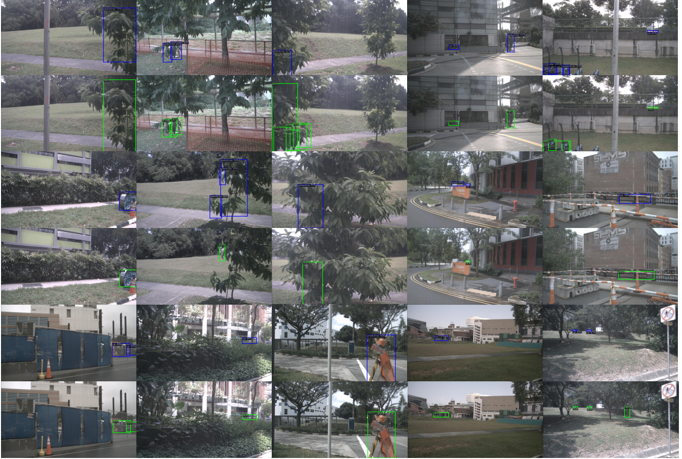
Figure 8. Additional visualization of detected objects on the OOD images (from nuImages) by a vanilla Faster-RCNN ( top ) and STUD ( bottom ). The in-distribution is BDD100K dataset. Blue : Objects detected and classified as one of the ID classes. Green : OOD objects detected by STUD, which reduce false positives among detected objects.
