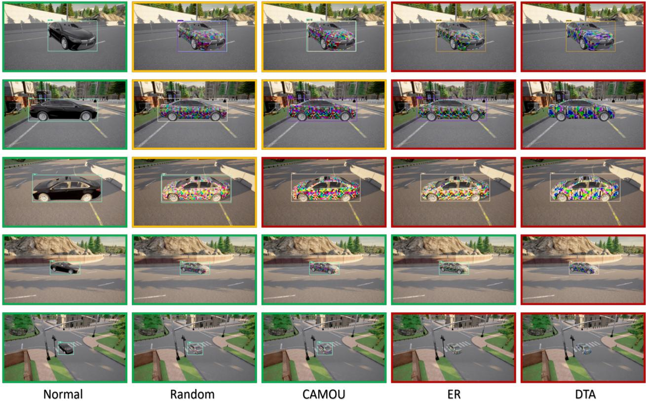
Figure 21. Sample images of adversarial camouflage on CARLA Simulator with different camera poses. Border: Red = miss-detection; Yellow = partially correct (other label also detected); Green = correct (detected as car).
