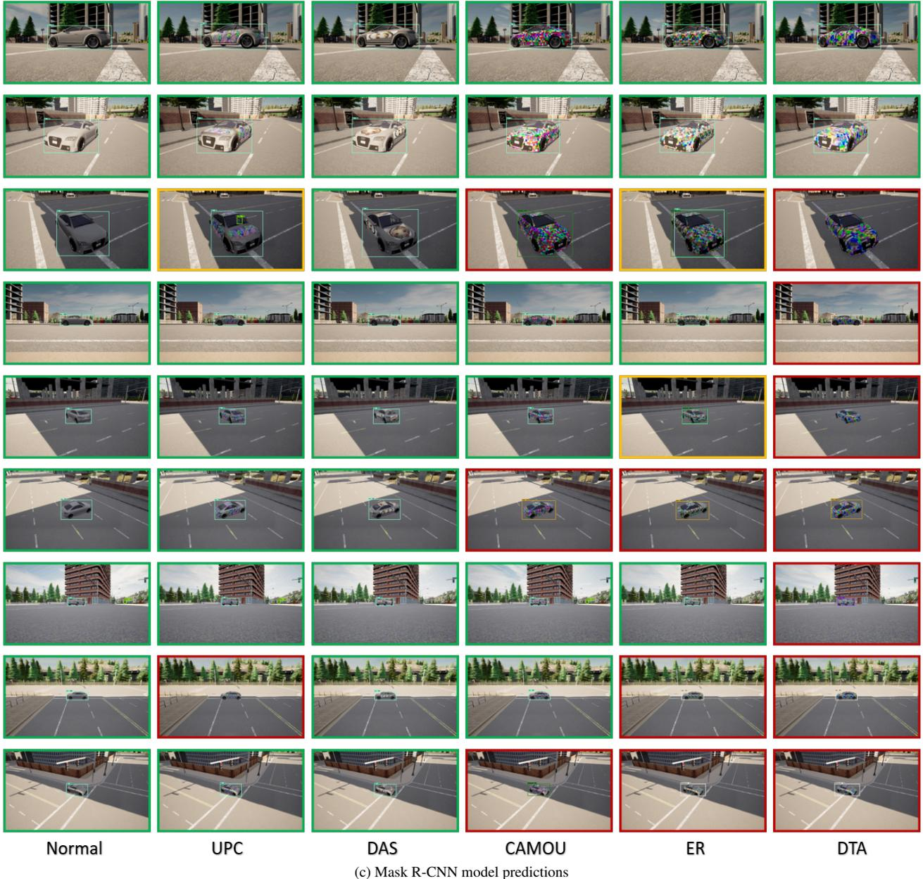
Figure 23. Transferability: Sample images of adversarial camouflage on CARLA Simulator with different camera poses. Border: Red = miss-detection; Yellow = partially correct (other label also detected); Green = correct (detected as car).
