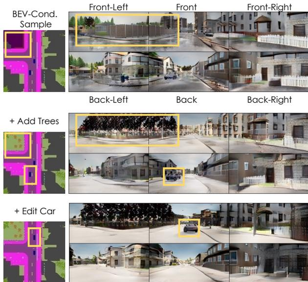
Figure 9. **BEV-Conditioned Synthesis**: NF-LDM allows controllable generation by editing the BEV segmentation map. From the initial sample, we add trees (green) and then edit the location of the car (blue). Note the ego car is at the center and thus not rendered.
