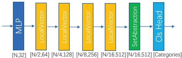
Figure 7. **The Classification architecture PointVector-S.** For comparison with PointNext [28], we replaced the SetAbstract module with the LocalVector module, keeping the other parameters the same.
