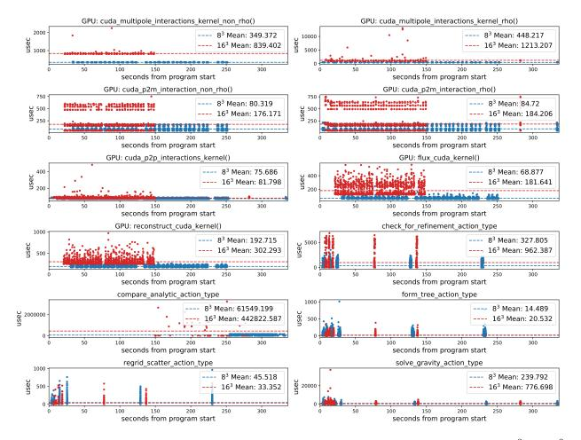
Figure 6: GPU kernel activity and CPU task actions for the gravity and hydro tasks when executing the  $8^3$  and  $16^3$  rotating star test on 6 localities. The  $16^3$  decomposition leads to longer-running tasks and kernels, but a shorter overall execution time because there are significantly fewer of them.
