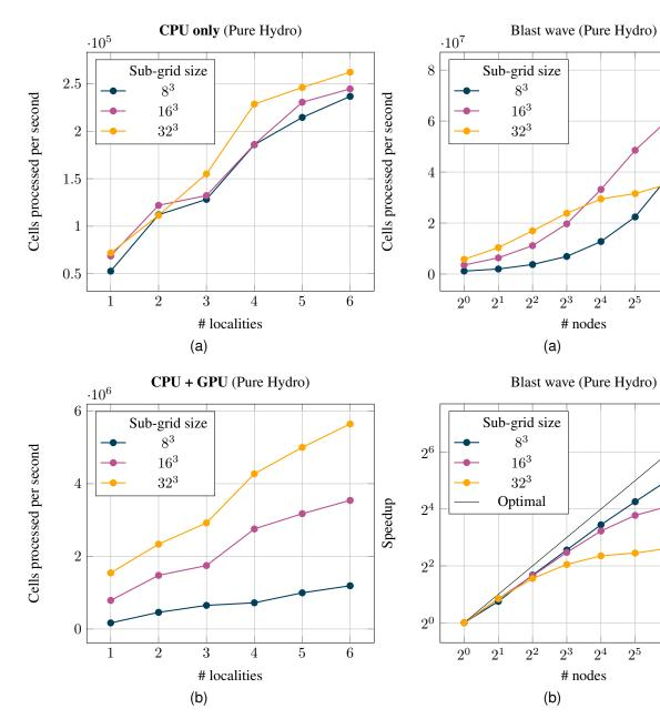
Figure 2: Cells processed per second for the node level scaling. For one up to 6 localities on one Summit node. One locality was assigned to seven CPUs and one NVIDIA V100 GPU.
