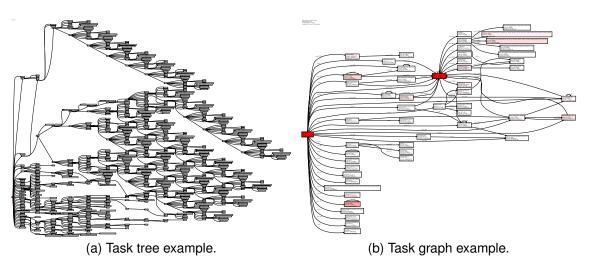
Figure 1: Task tree and task graph of Octo-Tiger as captured by APEX. Intensity of red color is correlated with the node's contribution to the overall runtime. The recursive structure of the octree is evident in the expanded tree. High resolution images are available here (https://doi.org/10.6084/m9.figshare.14666184.v1).
