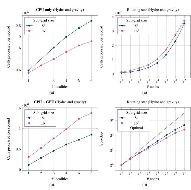
Figure 4: Cells processed per second for the node level scaling. For one up to 6 localities on one Summit node. One locality was assigned to seven CPUs and one NVIDIA® V100 GPU.
