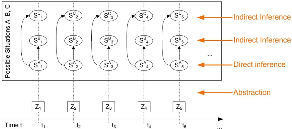
Fig. 3. Networks of situations, divided into directly and indirectly inferred situations.
