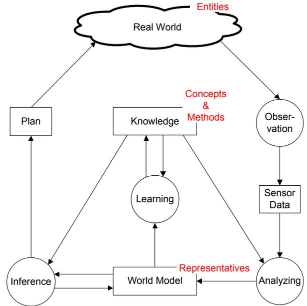
Fig. 1. Information flow and terminology in a surveillance system represented by information aggregates (boxes) and processes (circles).
