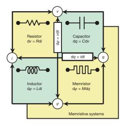
FIG. 4: The four fundamental two-terminal circuit elements, [14, p. 80]
