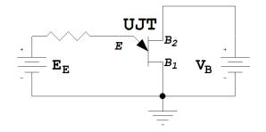
FIG. 2: Schematic structure of the UJT with the bias voltage.
