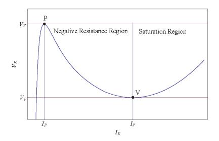
FIG. 3: Static Emitter Characteristic of the UJT.
