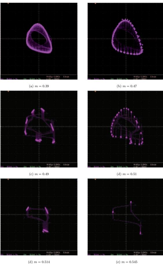
FIG. 10: Torus breakdown in the UJT circuit for various values m.
