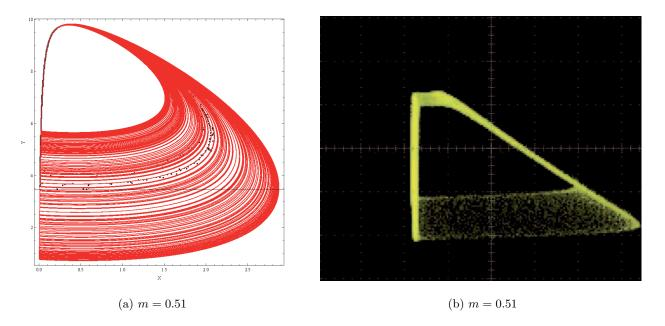
FIG. 9: Phase portrait of dynamical system (13) and oscilloscope snapshot of UJT circuit for m = 0.51.
