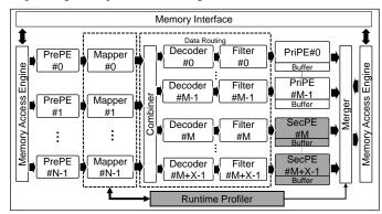
Fig. 3: The skew-oblivious data routing architecture. Modules in solid grey color are enqueued and dequeued dynamically.
